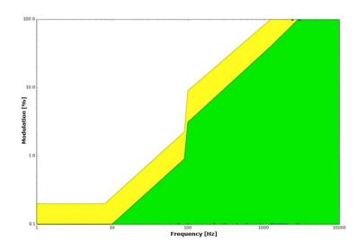
Thanks to the 4khz dimming frequency the MINI-1CV-DALI allows to reduce the Flicker phenomenon.
