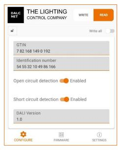
Through the Lamp-Failure command, the DALI protocol allows you to detect situations in which the LED load connected to the output of the MINI-1CV-DALI may not work as expected, such as an incorrect connection (detecting it as an Open Circuit error) or a defect in the LED load (detecting it as a short circuit).
